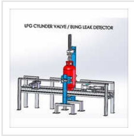
LPG Cylinder Valve Bung Lead Detector
