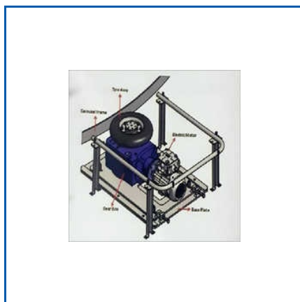
DRIVE UNIT LPG BOTTLING PLANT
